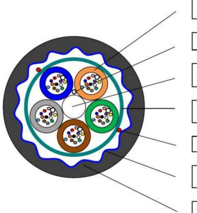
Loose tube with Optical fibers and water blocking yarn(s)
